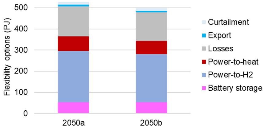
Figure 23. Use of excess electricity by flexibility options deployed in scenario 2050a and 2050b in PJ.
