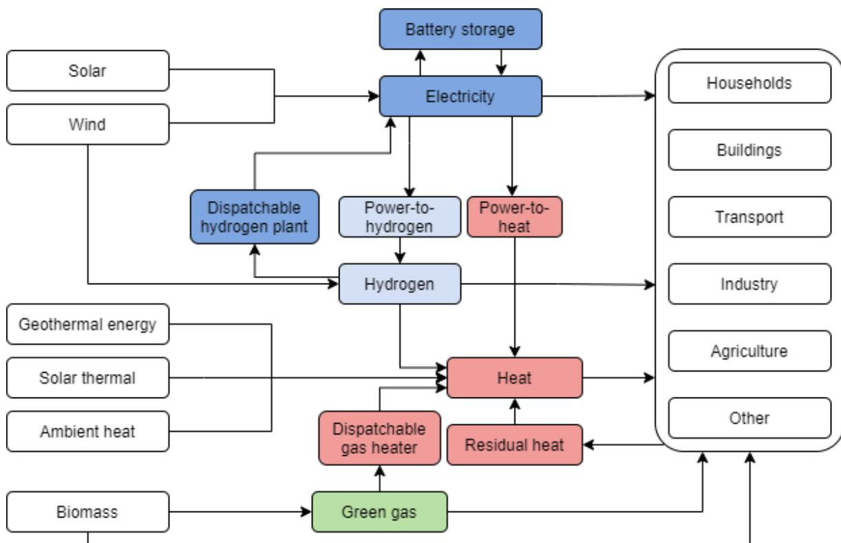
Figure 9. Schematic overview of the modelled energy system including the energy supply (left), flexibility options (middle), and the energy demand (right). The overview is highly simplified, and many components are left out for clarity purposes. Darker blue corresponds to the electricity component of the scenario, light blue to hydrogen, red to heat, and green to green gas.
