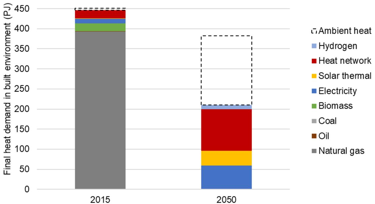
Figure 12. The final heat demand in the built environment in 2050 compared to 2015 in PJ.
