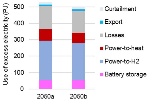
Figure 4. The use of excess electricity in 2050a/b (PJ).
