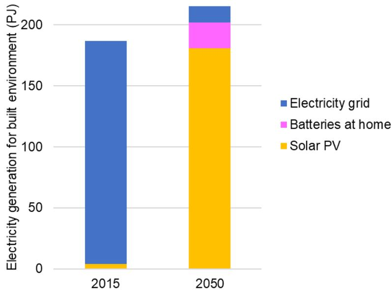
Figure 11. The final electricity demand for 2050 compared to 2015 in PJ per source of electricity generation.
