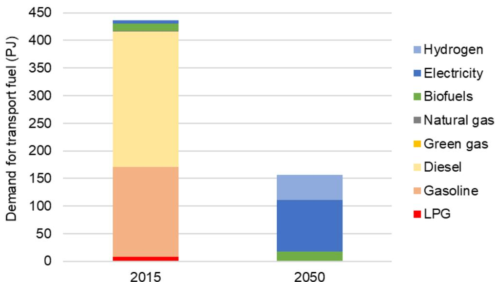
Figure 13. The energy carriers used as transport fuel for national transport in 2050 compared to 2015 in PJ.
